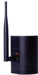
portable wireless distributed vibration test equipment
